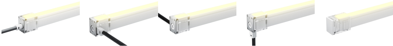
ARVO-M-MEC1-F-2P Mechanical end cap with screws, front entry with 0.98ft(30cm) cable, 2 pin ARVO-M-MEC1-LS-2P Mechanical end cap with screws, left side entry with 0.98ft(30cm) cable, 2 pin ARVO-M-MEC1-RS-2P Mechanical end cap with screws, right side entry with 0.98ft(30cm) cable, 2 pin ARVO-M-MEC1-B-2P Mechanical end cap with screws, bottom entry with 0.98ft(30cm) cable, 2 pin ARVO-M-MEC3-C Mechanical closed end cap without screws
