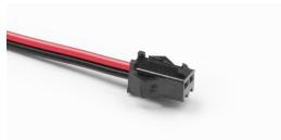
FC-2P-20 Female connector with 0.66ft (20cm) 2pin, IP20, 24AWG
